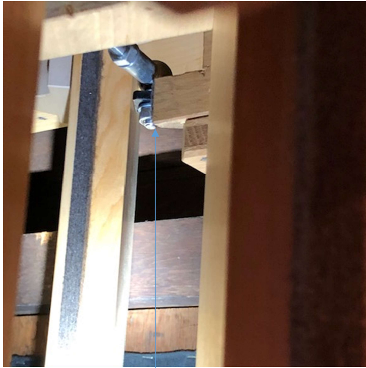
Wooden block with minimal felt causing banging in the Swell south shutter front mechanism. This would be shaved and a thicker felt installed to limit noise
