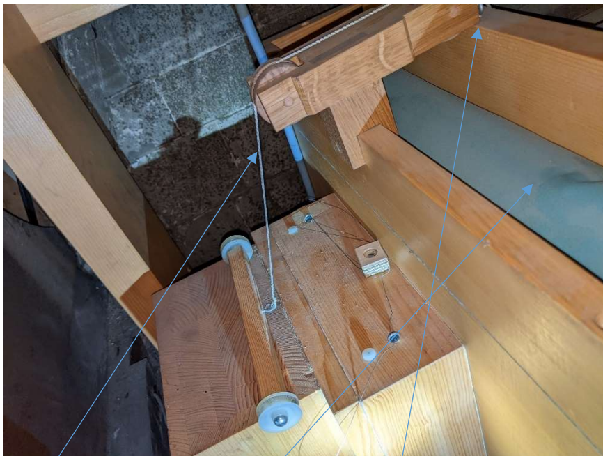
Pedal wind system. The roller blind is held open by the thin wire that can be seen in the middle of the photograph. The Schwimmer reservoir naturally inflates to the maximum with the rollerblind held open, so that the top part of the Schwimmer is hard against the top of the roller valve mechanism
