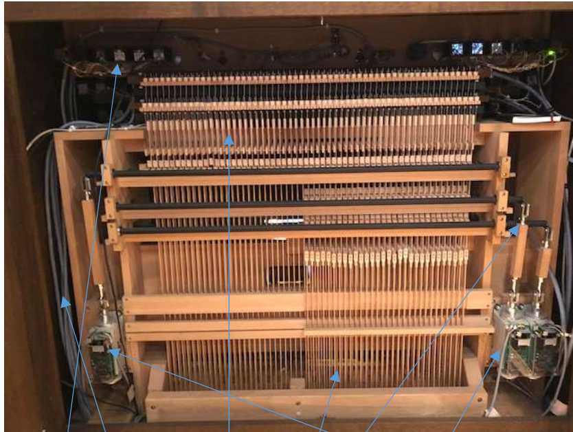
Behind the console. The manual and Pedal key and coupler actions, drawstop solenoids, wiring and robust coupler mechanisms and motors are all visible
